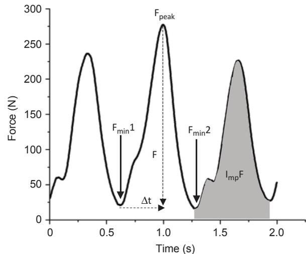
Figure 5. Determinant instants used for force-time curve analysis.  $F_{\text{peak}}$  = Peak force;  $I_{\text{imp}}F$  = impulse, represented by the curve's area;  $F_{\text{min}1}$  = beginning of the stroke;  $F_{\text{min}2}$  = end of the stroke;  $\Delta t$  = time variation;  $\Delta F$  = force variation.
