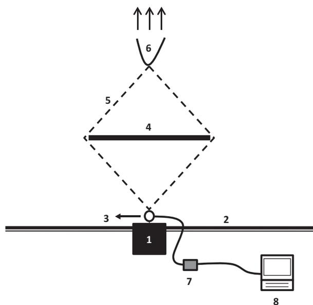
Figure 3. Top view of the tethered swimming: (1) starting platform, (2) wall, (3) load cell, (4) floating bar, (5) inextensible cables, (6) belt, (7) interface and (8) computer. Swimmers were instructed to swim according to the arrows' direction.
